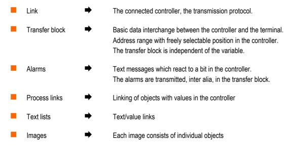
An interpreter works through the project in the terminal. This interpreter depends on the selection of the link. It constitutes the connection to the controller, with the corresponding protocol. The interpreter is transferred to the terminal together with the project.
