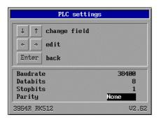
Some of these settings are dependent on the interpreter that is in use. If you use the S5-PG Mode interpreter, for instance, you cannot change the COM port settings, because they have been fixed by Siemens.
