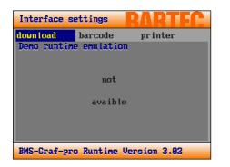
The run time emulation is used for starting up projects at exhibitions, trade fairs and demonstrations without SPS system. Addresses for a simulation are specified. These addresses are described in appendix A.
