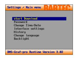
Settings during regular operation are achieved by pressing the "i" key. This is similar to the previous set up. If alarms are present these are first displayed. By repeated depression of the "i" key the set up is reached.
