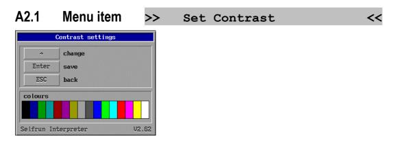
Press ➡ to change the contrast. While ➡ is being pressed, the PC display terminal will get darker at first, and then brighter again. As soon as you have reached the desired contrast, either press ENTER to save the current contrast value or ESC to revert to the original contrast settings.
