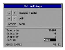
Enter here the COM port settings for a bar code scanner or a similar device (ASCII characters).
