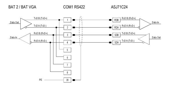
Make sure you use double-stranded cables only. The connections to the interface module must be given two terminating resistors.
