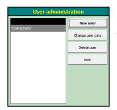
Users can be changed, deleted or created in the POLARIS Panel. This serves to adjust the system without the necessity of downloading again. Changes are limited to the POLARIS panel.
