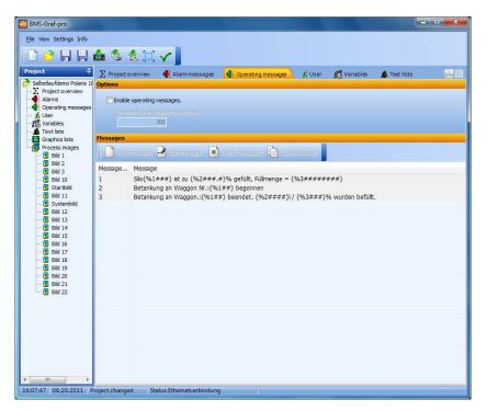
It is possible to process messages in the BMS-Graf-pro. A transfer range to the control is defined. It permits two types of operating messages:
