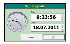
Accept writes the set values into the internal system clock module.
