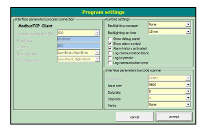
Depending on the setting in the BMS-Graf-pro project, the **process link interface parameters** can be altered. If changing is necessary, the settings on the device are saved separately and loaded on starting. If no change is possible, only the settings from the project are used. In this case, this dialogue only displays the parameters.
