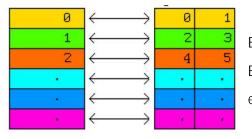
Byte 0 and byte 1 in memory are word address 0 Byte 2 and byte 3 in memory are word address 1 etc.
