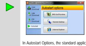
In Autostart Options, the standard application is selected which is to be started immediately and when the device is next booted. The settings in the applications (Remote Desktop and Internet Explorer) must be parameterised in the corresponding program-specific option.
