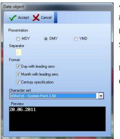
"Date object" dialog window for the current date on the internal clock in the POLARIS Panel.
