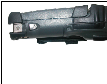
Figure 5: Keypad mounted correctly
