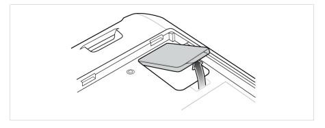
5. Position of the nano-SIM slot in the TC26ex-NI.
