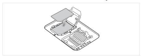
9. Close the nano-SIM card holder door and slide to the lock position.
