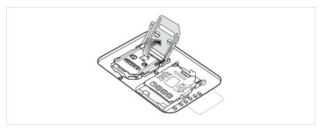
8. Place the nano-SIM card into the card holder with contacts facing down.
