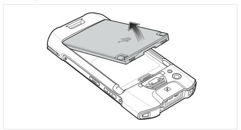
8. Insert the replacement battery, bottom first, into the battery compartment in the back of the device.
