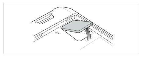
5. Slide the microSD card holder to the Open position.
