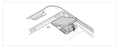
11. Access door must be replaced and tightened to provide an adequate seal for the device.
