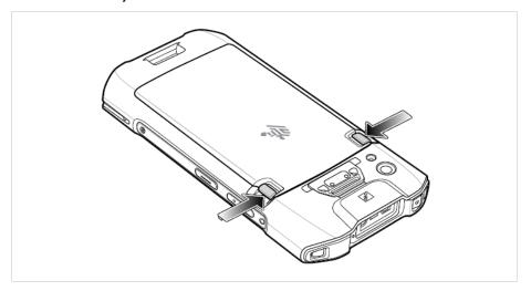
7. Lift the battery from the device.
