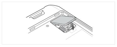
10. Access door must be replaced and tightened to provide an adequate seal for the device.
