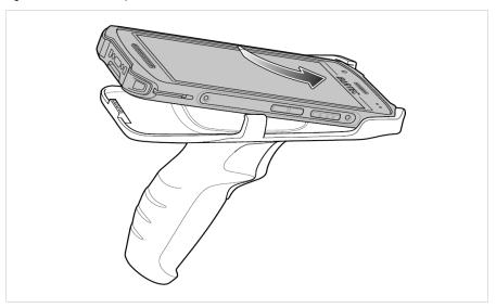
3. Rotate the device down and press down until it snaps into place.
