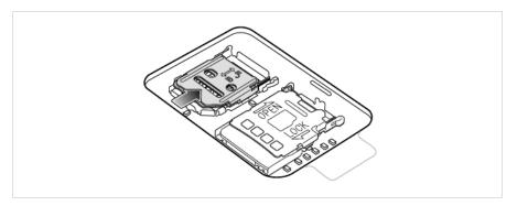
6. Slide the nano-SIM card holder to the unlock position.
