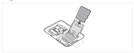
8. Close the microSD card holder door and slide the door to the Lock position.
