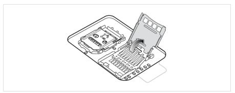
7. Insert the microSD card into the card holder door ensuring that the card slides into the holding tabs on each side of the door.
