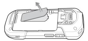
3. Insert the microSD card into the card holder door ensuring that the card slides into the holding tabs on each side of the door.
