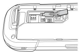
Figure 3 Mini SIM Card Installation
