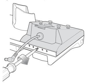
9. Align mounting holes on the bottom of the Four Slot Battery Charger with the stubs on the Battery Adapter.
