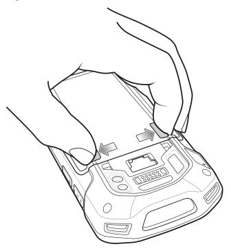
6. Lift the battery from the device.
