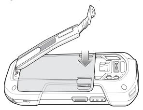
5. Place hand strap clip into hand strap mounting slot and pull down until it snaps into place.
