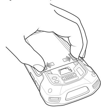
8. Lift the battery from the device.
