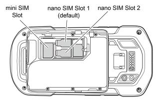
2. Insert a SIM card into the SIM slot with the cut edge toward the middle of the device and the contacts facing down.
