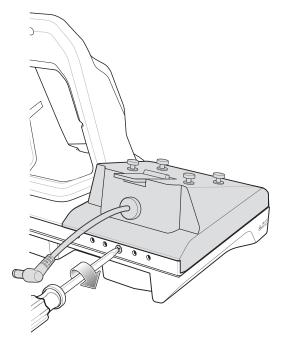
9. Align mounting holes on the bottom of the 4-Slot Battery Charger with the stubs on the Battery Adapter.
