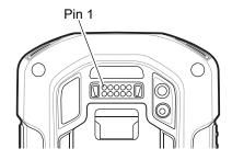
Figure 151 I/O Connector
