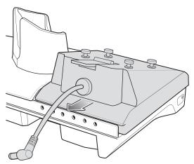
8. Using a Phillips screwdriver, secure adapter to cradle base with screw.
