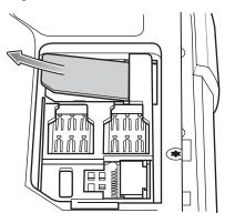
Figure 19 Remove Nano SIM Card
