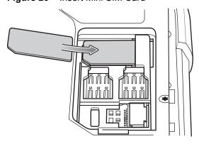
Figure 21 Insert Nano SIM Card
