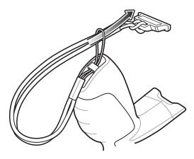
3. Pull the attachment plate until the loop tightens on the tether.
