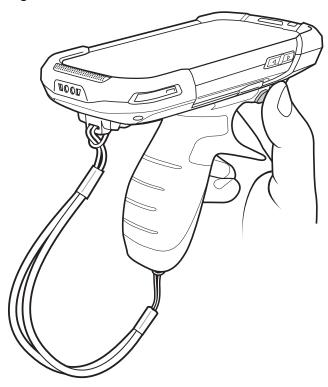
2. Rotate the device up and remove from the Trigger handle.
