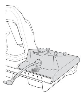
8. Using a Phillips screwdriver, secure adapter to cradle base with screw.
