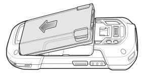
2. Press the battery down into the battery compartment until the battery release latches snap into place.
