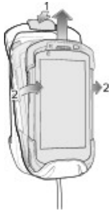
Figure 59 Remove Device from Cradle
