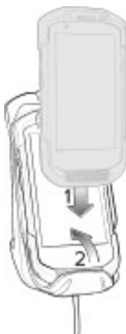
Figure 58 Insert Device into Cradle
