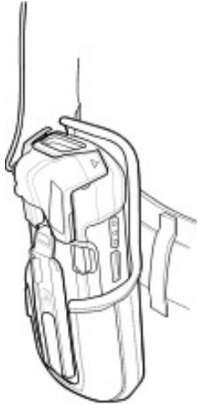
Figure 52 Device with 3.5 mm Audio Adapter in Holster
