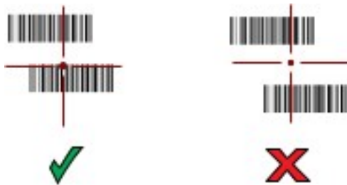
Figure 24 RS5100 Pick List Mode with Multiple Barcodes in Aiming Pattern
