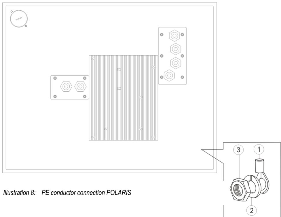
Illustration 8: PE conductor connection POLARIS
