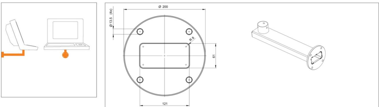
Illustration 5: Drilling pattern - supporting system for wall mounting
