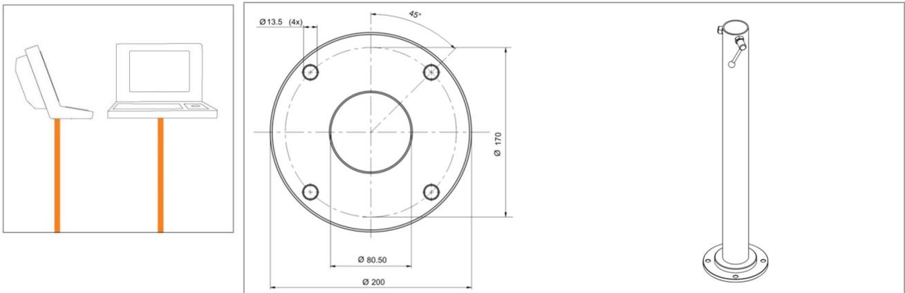
Illustration 4: Drilling pattern - supporting system for floor mounting
