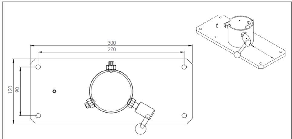
Illustration 6: Drilling pattern - supporting system for table mounting
