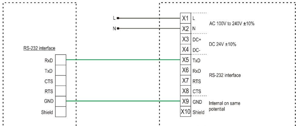
**6.7.5 Replacement 160ex with connector to Universal Power Supply Exi**
