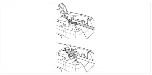
3. Feed the connection cable through the cable gland.
