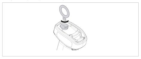
2. If a battery has been inserted: remove the battery.
