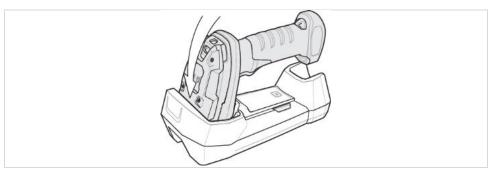
2. Press the underneath of the hand-held scanner into the base station until you hear the hand-held scanner click into place.
