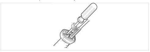
4. Push the safety lock into the closed position.
