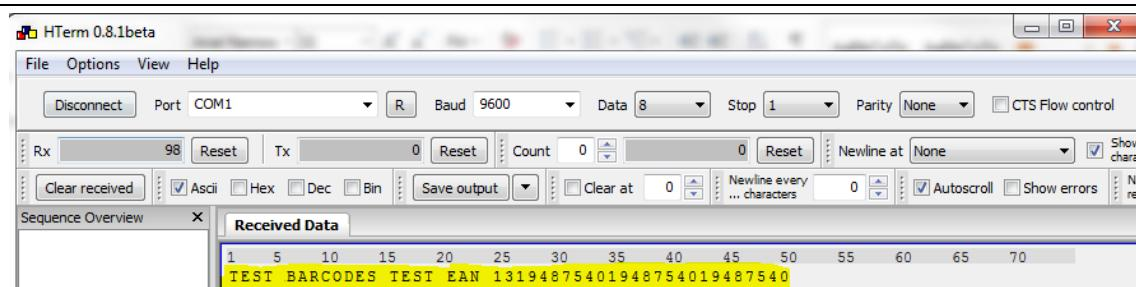
Data transmission is OK if the barcode data is displayed in the "Received Data" window.
