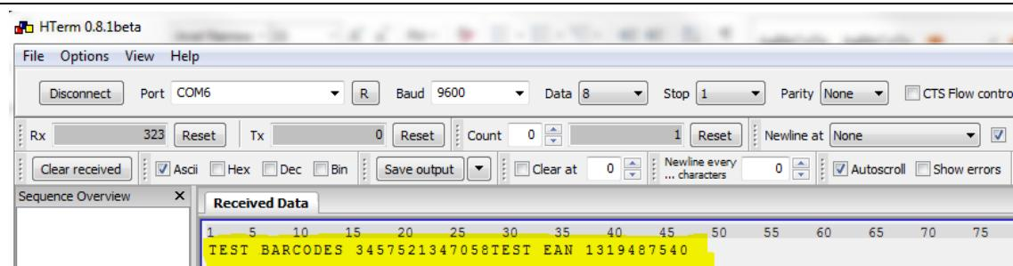
Data transmission is OK if the barcode data is displayed in the "Received Data" window.
