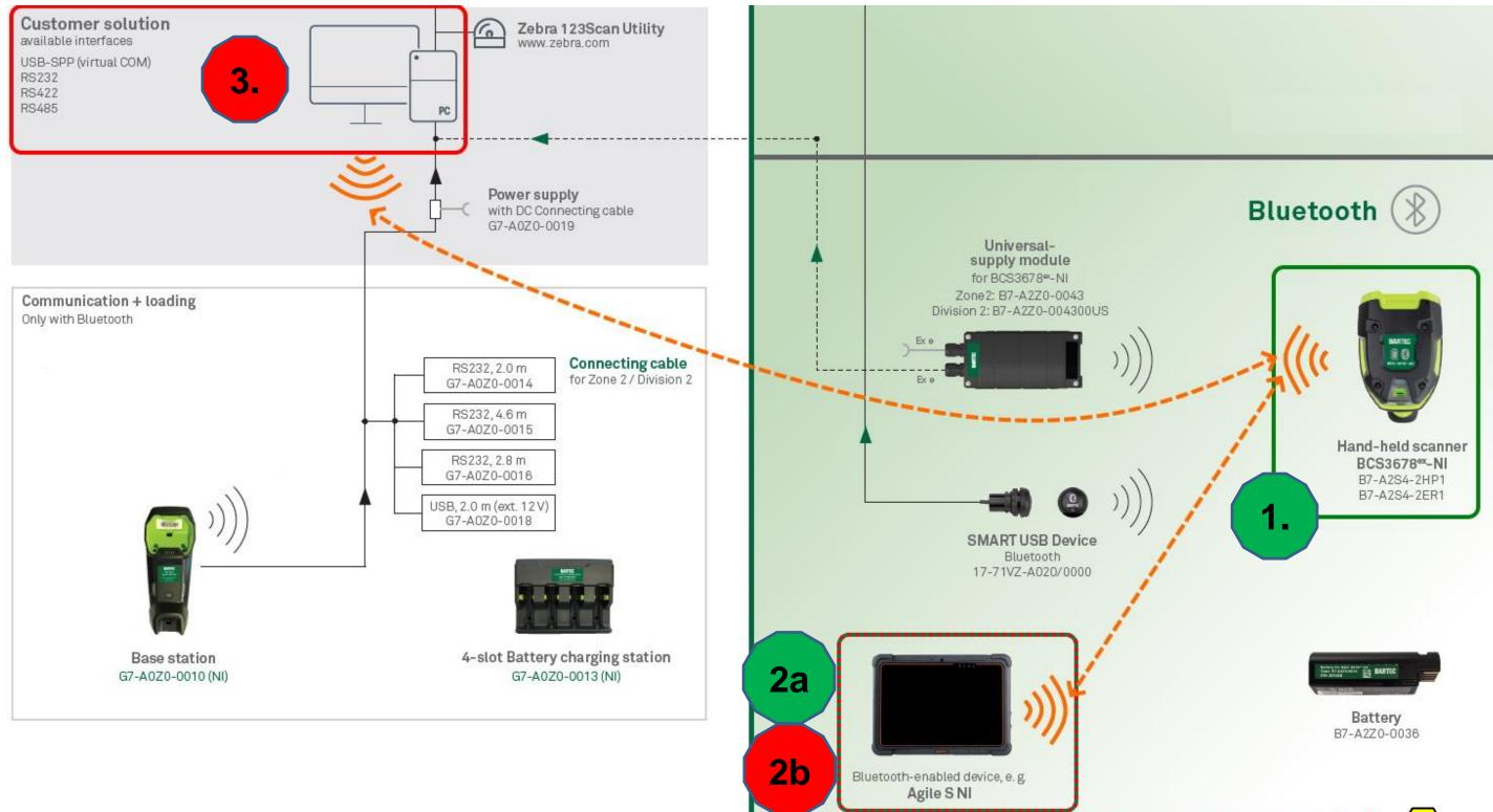
Green = Components from BARTEC for use in hazardous location Zone 2/22 or Division 2 Red = Customer-specific components (not supplied by BARTEC)
