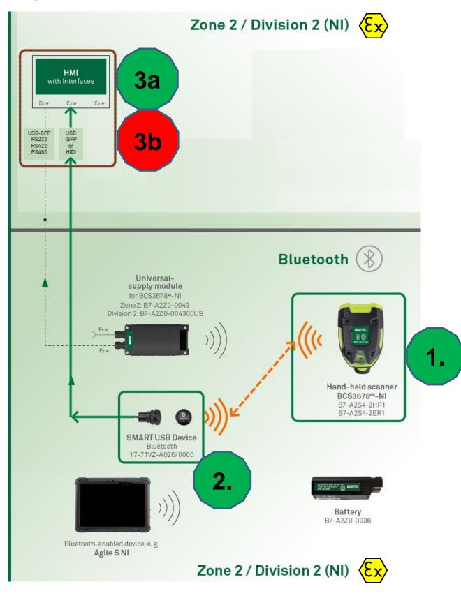
Green = Components from BARTEC for use in hazardous location Zone 2/22 or Division 2 Red = Customer-specific components (not supplied by BARTEC)
