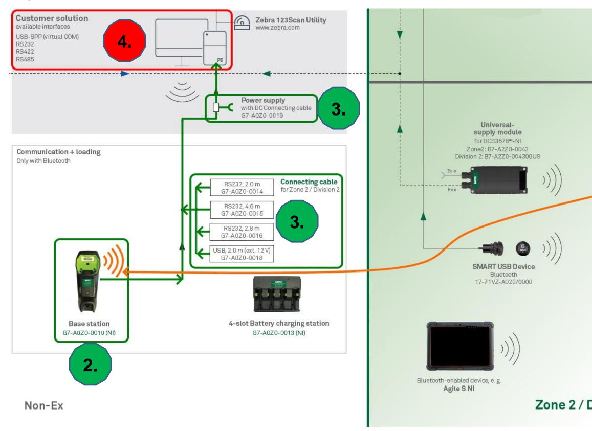
Green = Components from BARTEC for use in hazardous location Zone 2/22 or Division 2 Red = Customer-specific components (not supplied by BARTEC)
