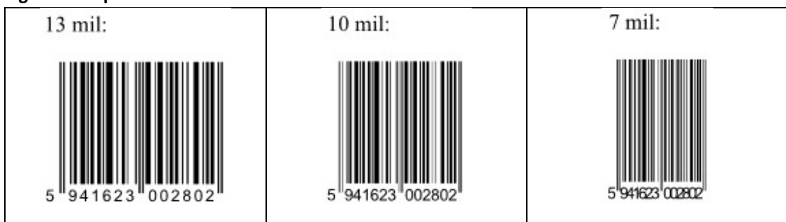
Fig. 4: Example of barcode sizes in mil
