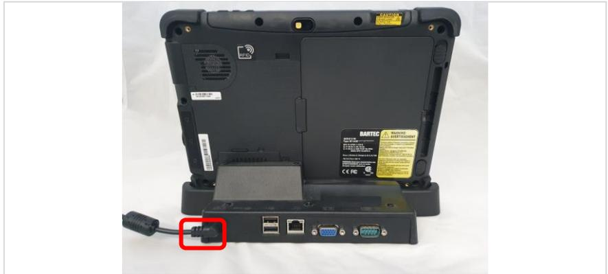
2. Plug the standard non-Ex USB stick with the operating system into a USB port of the docking station.
