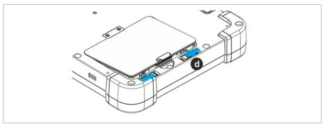
5. Press the battery/cover module into the battery compartment (e).
