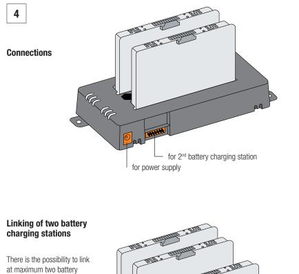
Charging stations There is the possibility to link at maximum two battery charging stations charging them with only one power supply.
